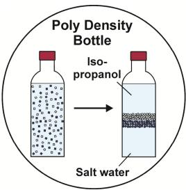
completely separated into salt water and isopropanol and the two layers of beads meet at the resulting isopropanol-saltwater interface.
